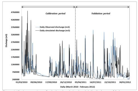
Figure 4.12: A comparison of calculated and simulated daily discharge of Rukarara catchment, south west Rwanda (March, 2010 - February, 2012)
