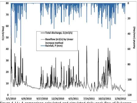
Figure 4.11: A comparison calculated and simulated daily peak flow of Rukarara catchment, south west Rwanda (March, 2010 - February, 2012)
