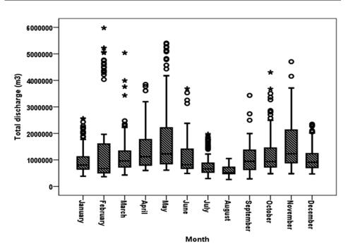
Figure 4.9: Variability of mean monthly discharge over 3 years (March-2010 to February 2013). The box-and-whisker diagrams include: median value; (large rectangle) range of 50% of the samples; (cross bars)
