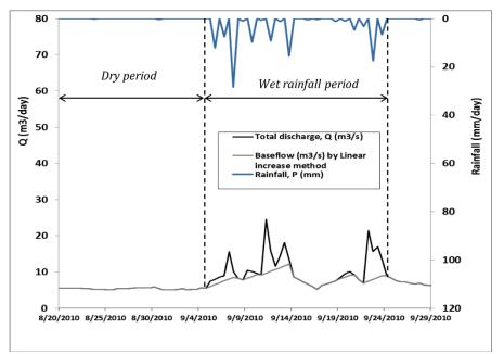
Figure 4.10a: Example of base flow separated from the discharge by simple linear increase (equation 21) during the dry and rainy periods of Rukarara catchment, south west Rwanda
