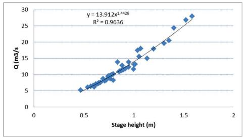
Figure 4.8: Stage-discharge calibration curve for the Rukarara catchment, outlet station
